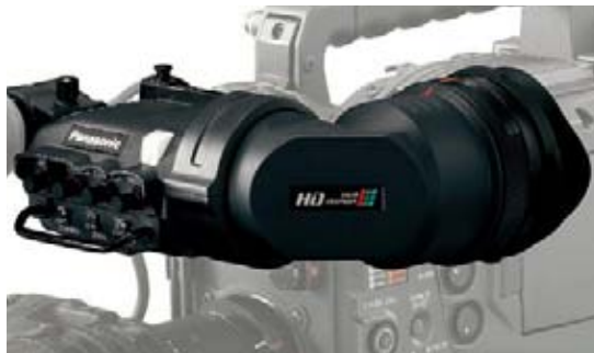
AJ-CVF100G 25.4 mm (1 inch) HD Color EVF Utilizing a 25.4 mm (1 inch) LCOS (Liquid Crystal On Silicon) display panel, the AJ-CVF100G provides cinematographers with accurate colors, fast motion response, excellent resolution, and smooth pixel edges for a natural look and feel, which minimizes the possibility of misdirected shots.
