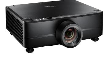
At 9,800 lumens with 4K and HDR compatibility, the ZU920T features a dust-resistant IP5X certified optical engine for 24/7 operation
