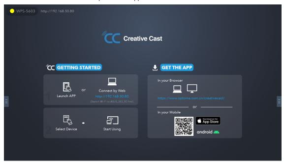
Note: For initial activation of the iOS screen mirroring function, please ensure the projector is connected to the internet, then launch the Creative Cast app. You are only required to perform this initial step once and after the initial connection is established, the Creative Cast app does not need to be open for future use of the iOS screen mirroring function.
