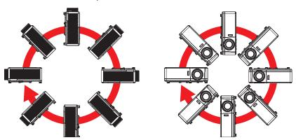
Allow at least 30 cm clearance around the exhaust vent.
