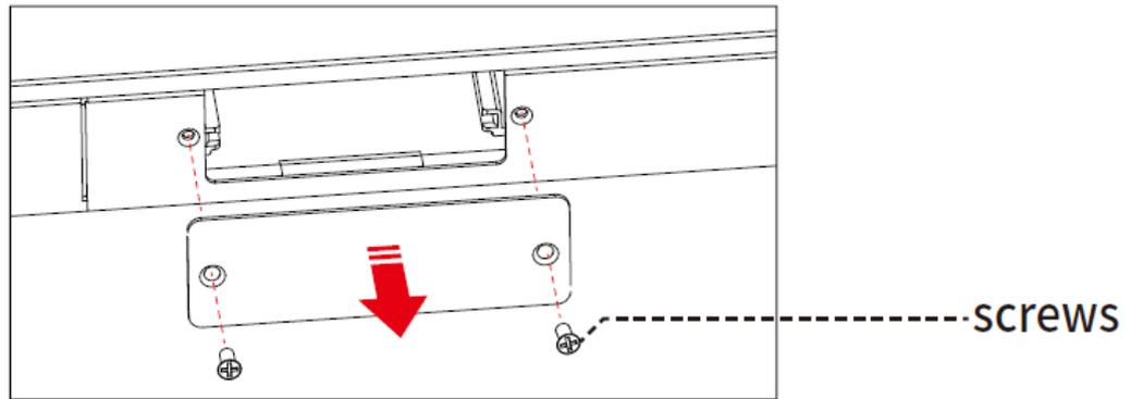
**Step 2** Insert the SDM-S into the port on the rear of the panel until firmly seated, using the 2 screws to secure it.
