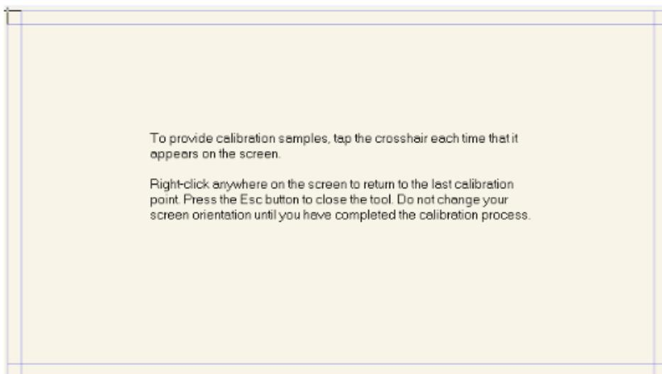
**Step 7** After the calibration is complete, the **Digitizer Calibration Tool** dialog box will be displayed. Click **Yes** to save calibration data.
