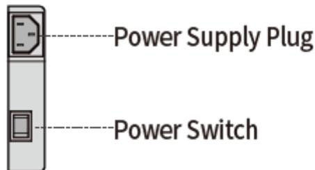
**Step 3** Press the power button
