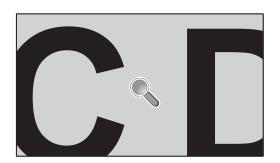
The [POINT ZOOM] function increases the image size and expands it horizontally and vertically simultaneously. The image can be increased up to 10 times its size.
