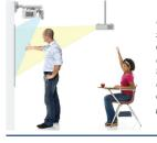
Ultra short throw creates a 77" standard or 87" widescreen diagonal image from a mere 23 inches, eliminating shadows on the screen along with projected light in the presenter's eyes created by traditional front projection systems.
