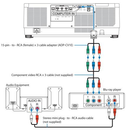
• Select the source name for its appropriate input connector after turning on the projector.
