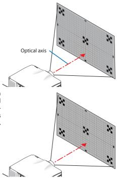
Press ▼ button to select the [PERIPHERY] on the on-screen menu, and then press either ◄ or ▶ button to align the focus of screen peripheral area. During this operation, the focus for around the optical axis will be maintained.
