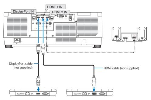
• Select the source name for its appropriate input connector after turning on the projector.
