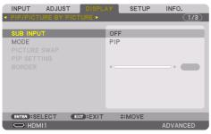
This displays the [PIP/PICTURE BY PICTURE] screen in the on-screen menu.
