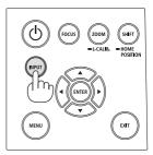
Press the ▼/▲ buttons to match the target input terminal and then press the ENTER button to switch the input. To delete the menu display in the [INPUT] screen, press the MENU or EXIT button.
