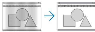
CLOCK Use this item to fine tune the computer image or to remove any vertical banding that might appear. This function adjusts the clock frequencies that eliminate the horizontal banding in the image. This adjustment may be necessary when you connect your computer for the first time.
