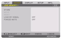
This function serves to store the adjusted values for each input signal when using the [LENS SHIFT], motorized [ZOOM], and motorized [FOCUS] functions of the projector. Adjusted values can be applied to the signal you selected. This will eliminate the need to adjust lens shift, focus, and zoom at the time of source selection.
