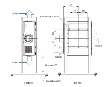
\*\* The example shows the right side of the body (side where the control unit is located) facing downwards. To make the left side of the body (side where the label is pasted) face downwards, leave a space of 200 mm or more.
