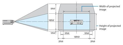
Description of symbols: V indicates vertical (height of the projected image), H indicates horizontal (width of the projected image).
