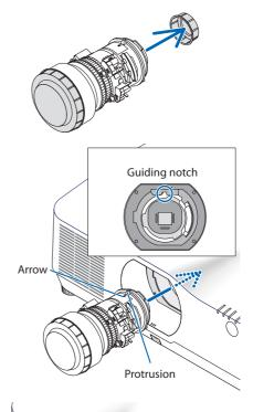
3. Insert the lens onto the projector facing the arrow on the lens-label upward.
