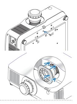
• Attach the enclosed lens mask if you want to hide the gap between the projector and lens.
