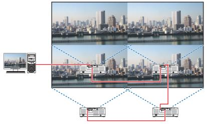
When performing settings or adjustments using one remote control, enable the [CONTROL ID] for assigning ID to each projector so as not to activate the other projectors. ( $\rightarrow$  page 138)
