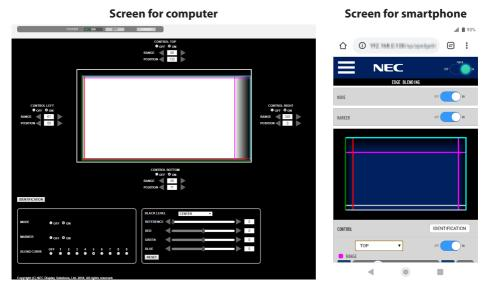
The [EDGE BLENDING] setting/adjustment items are displayed on one screen and can be operated using the mouse of the computer or the touch screen of the smartphone. For details of each setting/ adjustment, refer to the On-Screen Menu explanation.
