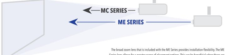
Series lens allows for a greater range of placement options. This can be beneficial when there are obstructions in the ceiling or when attempting to utilize existing screens, mounts and cable runs. A broad zoom lens can reduce installation costs and ensure sharp images that fill the screen properly.
