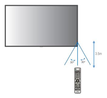
**NOTE**: The remote control system may not function when direct sunlight or strong illumination strikes the remote control sensor, or when there is an object in the path.
