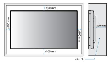
NOTE: • Allow adequate ventilation or provide air conditioning around the monitor, so that heat can properly dissipate away from the unit and the mounting equipment; especially when you use monitors in a multiple screen configuration.
