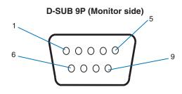
This monitor uses RXD, TXD and GND lines for RS-232C control.
