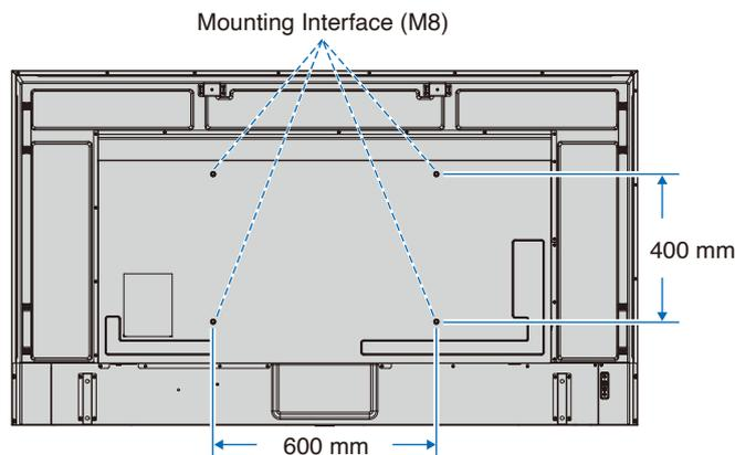
Mounting accessories can be attached with the monitor in the face down position. To avoid scratching the LCD panel, always place a soft cloth, such as a blanket that is larger than the monitor's screen area, on the table before laying the monitor face down. Make sure there is nothing on the table that can damage the monitor.
