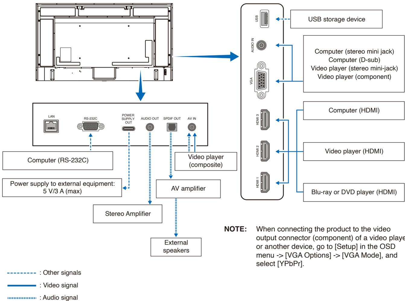
**NOTE:** When connecting the product to the video output connector (component) of a video player or another device, go to [Setup] in the OSD menu -> [VGA Options] -> [VGA Mode], and select [YPbPr].
