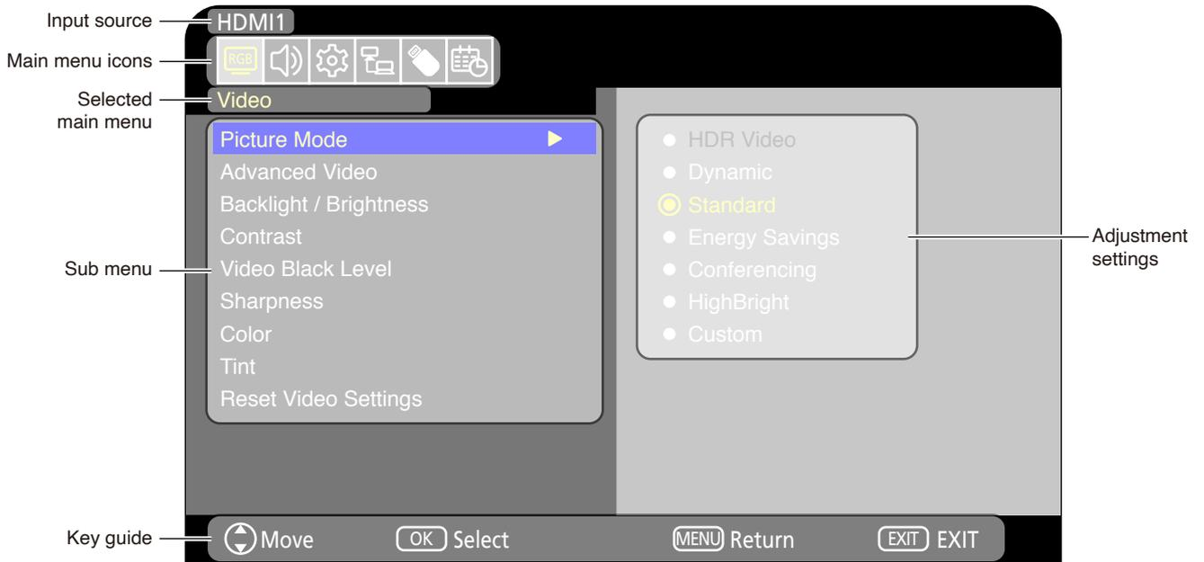
Press MENU to open and close the OSD menu. Press the EXIT button to close the OSD menu and stop OSD operations.
