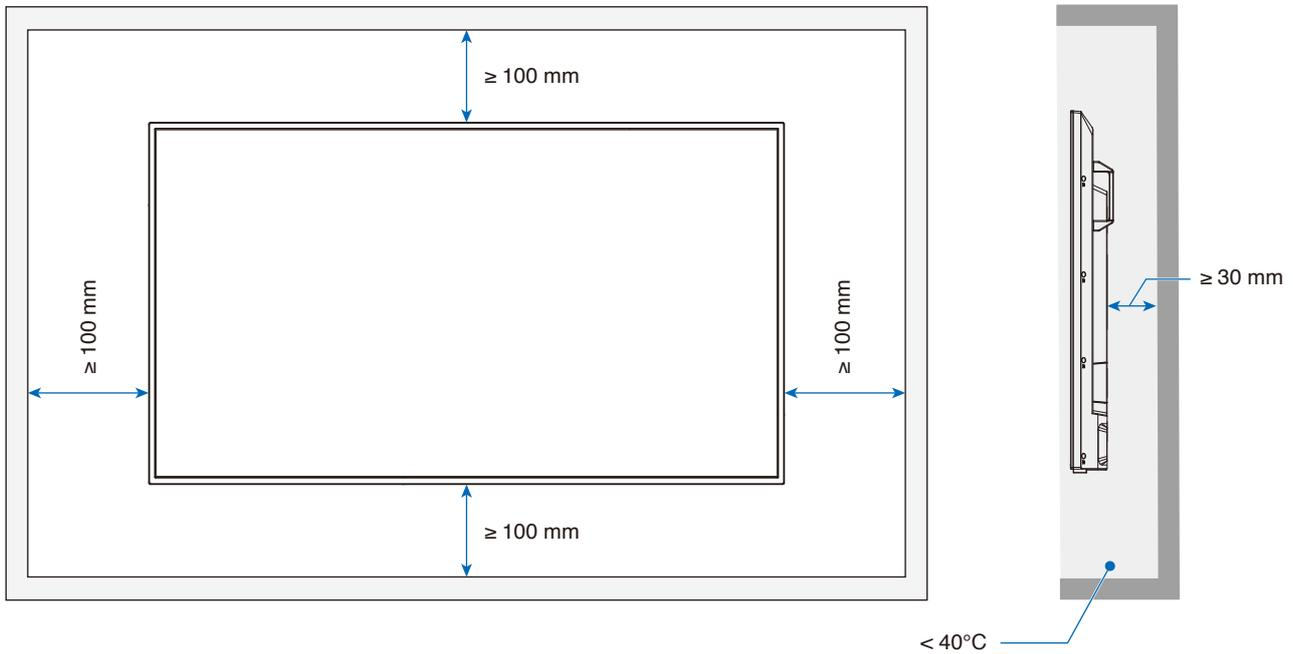
**NOTE:** The maximum environmental operating temperature of the monitor is  $40^\circ\text{C}$ . This monitor has internal temperature sensors.
