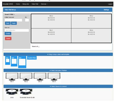
Figure 259: Video Wall Tab - Connecting Sources to Receivers
