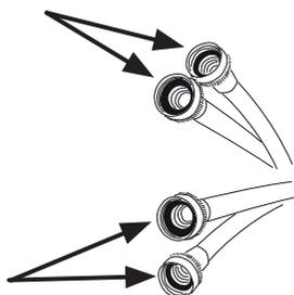
2. Tighten the hose and faucet fittings by hand until they are snug, then tighten them an additional two-thirds of a turn with pliers or a wrench. Pull the water supply hoses downwards to make sure that they are connected securely.
