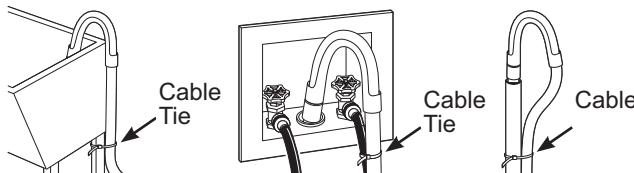
**NOTE:** Placing the drain hose too far down the drain pipe can cause a siphoning action. No more than 7 inch (17.78 cm) of hose should be in the drain pipe. There must be an air gap around the drain hose. A snug fit can also cause a siphoning action.
