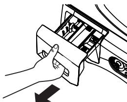
You may see water in the dispenser drawer at the end of the cycle. This is a result of the flushing/siphoning action and is part of the normal operation of the washer.
