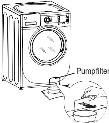
1. Using a coin or flat screwdriver in the notch on the door, open the access door.
