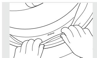
3. When you are finished cleaning the door gasket, remove your hands and the gasket will return to the operating position.
