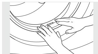
2. While holding down the door gasket, inspect the interior gasket by pulling it down with your fingers. Remove any foreign objects if found trapped inside this gasket. Make sure there is nothing blocking the holes behind the gasket.
