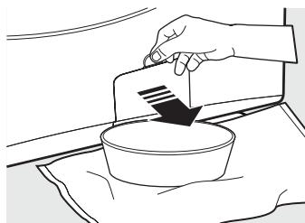
2. Place a shallow pan or dish under the pump access door and towels on the floor in front of the washer to protect the floor. It is normal to catch about a cup of water when the filter is removed.
