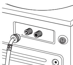
**Do not crossthread or over-tighten these connections.**
