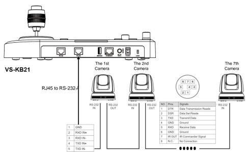
1. Please refer to the RJ-45 to RS-232 and camera Mini Din RS-232 pin definitions to complete the cable connection
