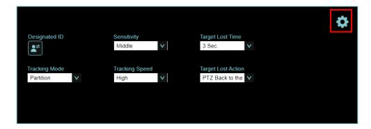
to enable the Partition edit, click the left mouse button to frame it (orange frame) in the panoramic preview window, determine the area and click to save. The partition icon below will be changed to the saved position
