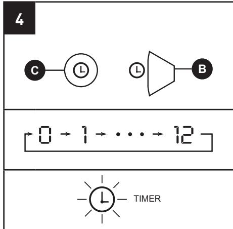
5. To set the timer to power on the heater, first ensure the unit is powered off, then press the timer button on the control panel (C).
