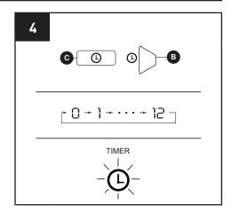
To set the timer power on, start the unit and press the Timer button on the control panel (C) or remote control (B).
