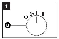
Set the thermostat by turning the thermostat knob on the control panel (B). You will hear a faint click when the unit's elements engage.
