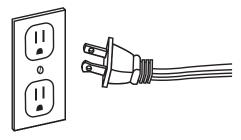
**A** WARNING: It is normal for the power cord to feel warm to the touch. However, a loose fit between the outlet and the plug may cause overheating of the plug. If this occurs, try inserting the plug into a different outlet. Contact a qualified electrician to inspect the original outlet for damage.
