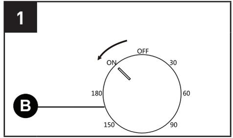
2. Set the timer OFF function by turning the knob clockwise to the desired time in minute in 30 min intervals between 30 to 180 minutes..
