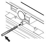
**12.** Drill through the outer steel sheet of the door through the holes shown below.
