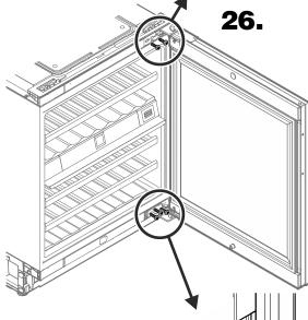
Adjusting the lateral tilt of the door
