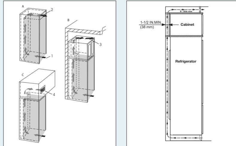
This type of cabinet must be carefully constructed using the correct dimensions and it must provide suitable ventilation to ensure proper appliance operation.
