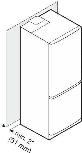
If the gap between the rear of the appliance and the wall is less than 2 inch (51 mm), the power consumption level may increase.
