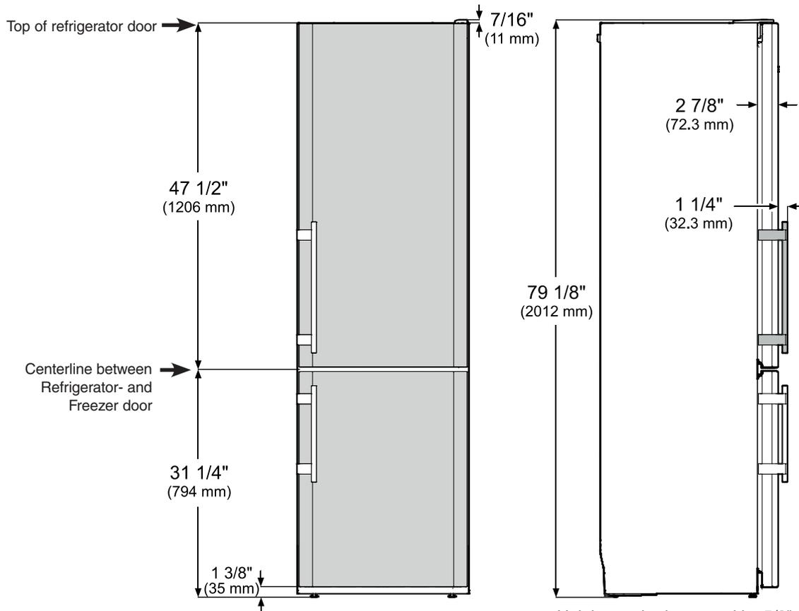
Height can be increased by 5/8" (16 mm) by turning the levelling feet at the front and the height adjustable roller units at the appliance rear.
