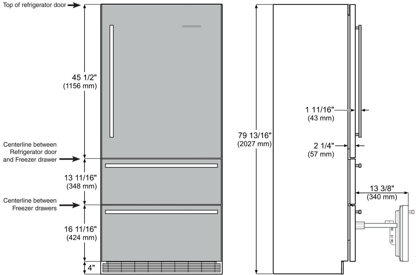
Height can be increased by 1-1/2" (40 mm) by turning the levelling feet at the front and the height adjustable roller units at the appliance rear.
