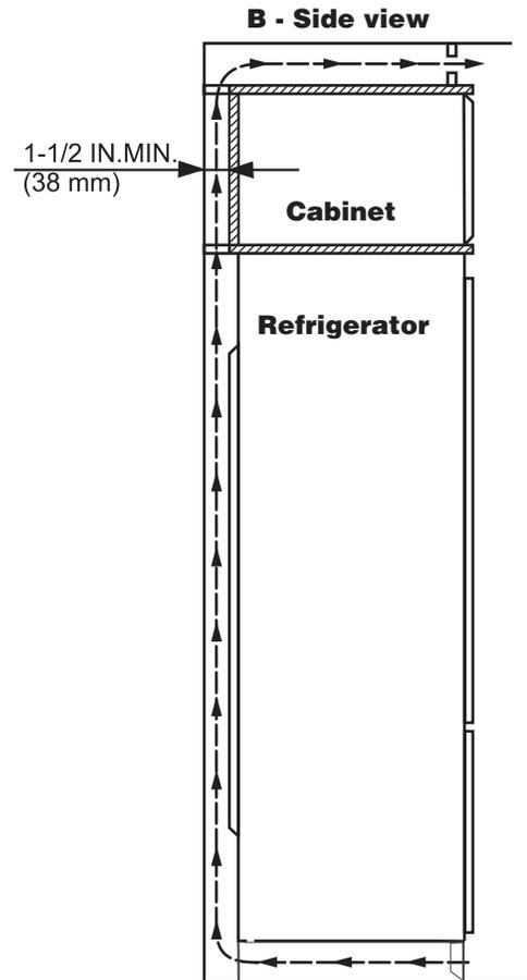
The refrigerator is designed to allow proper air flow when the appliance is installed up against the wall.
