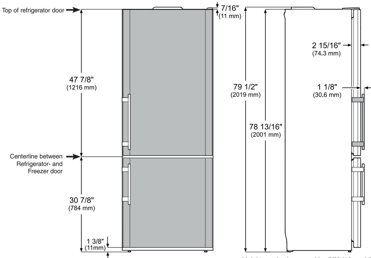
Height can be increased by 5/8" (16 mm) by turning the levelling feet at the front and the height adjustable roller units at the appliance rear.
