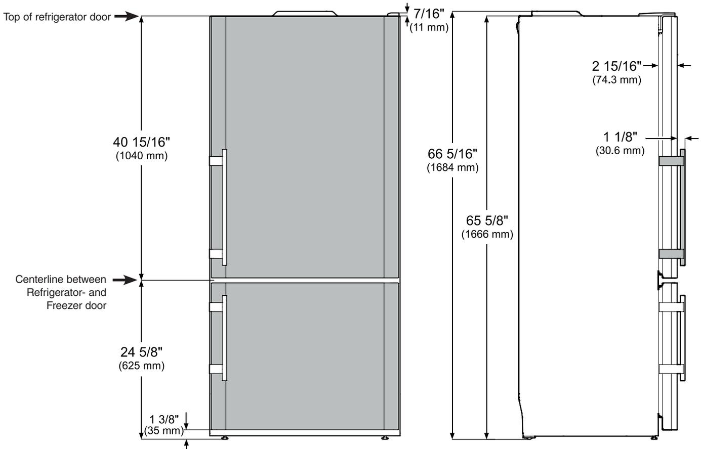
Height can be increased by  $5/8''$  (16 mm) by turning the levelling feet at the front and the height adjustable roller units at the appliance rear.
