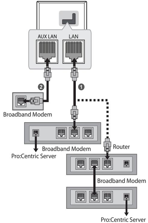
**1** Connect the **LAN** port of the Modem or Router to the **LAN** port on the TV.
