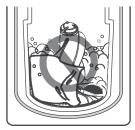
Do not load bulky items such as pet beds that are too large or stiff to move easily around the agitator. Impeding the motion of the drum or agitator could cause damage to the items or the washer.
