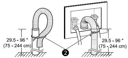
**Using a Standpipe to Drain**
