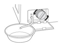
Clean the pump filter and opening.
