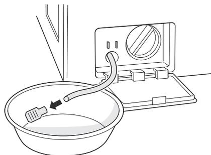
**4** Remove the pump filter.
