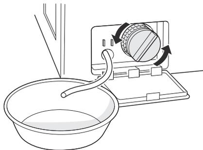
**5** Clean the pump filter and opening.
