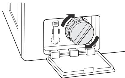
**8** Close the drain pump filter cover.
