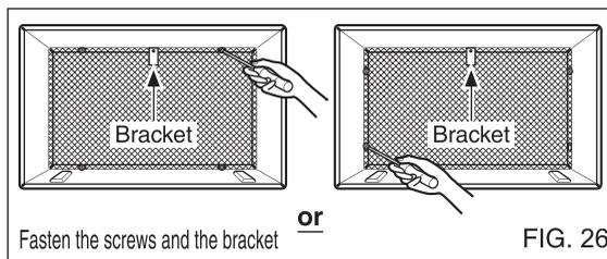
Fasten the screws and the bracket
