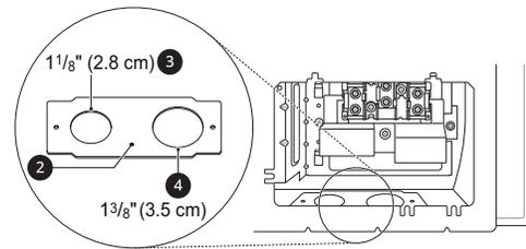
For power cord **5** installations, hook the strain relief over the 1 3/8 in. (3.5 cm) power cord hole located below the rear of the oven. Insert the power cord through the strain relief and tighten it.
