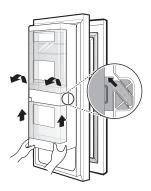
Pull out the crisper to full extension, lift the front up, and pull straight out.
