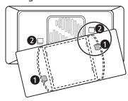
Rotate the air filter cover clockwise until the hooks engage and the cover locks in place.
