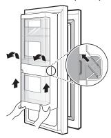
To replace the case, line up the tabs on the case with the slots on the door and push down until it snaps into place.
