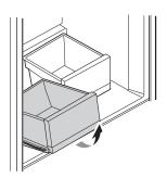
To reassemble, slightly tilt up the front, insert the crisper into the frame and push it back into place.
