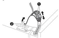
Rotate the hinge lever 3 counterclockwise. Lift the top hinge **4** free of the hinge lever latch **⑤**.
