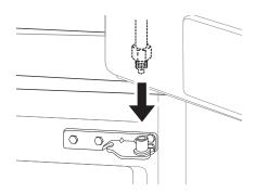
Fit the hinge **1** over the hinge lever latch **2** and slot it into place. Rotate the lever 3 counterclockwise to secure the hinge.
