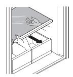
Pull out the crisper to full extension, lift the front up, and pull straight out.
