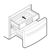
Replace the ice bin in the drawer. Insert the Durabase basket in the rail assembly.
