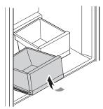
Insert the cover into the refrigerator with both hands and lower it onto the guides.
