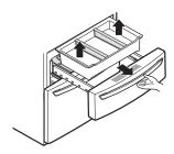
**2** Hold both sides of the door and remove it from the rails.
