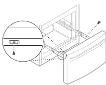
Insert the drawer into the frame, and push the drawer back until it clicks into place.
