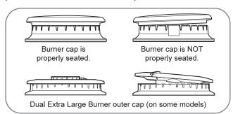
To place the dual extra large burner outer cap properly, make sure the slit in the burner cap is positioned over the assemble guide in the burner head.
