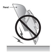
2 If the product is tilted onto the edge of the panel, the panel may be damaged.
