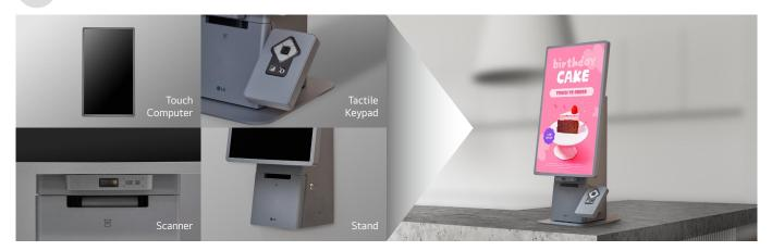
The Kiosk offers flexible customization with various peripherals to meet specific needs. Its modular design allows easy integration of devices like barcode scanners and EMV terminals. USB-C ports simplify connections, enabling independent operation for diverse business requirement.
