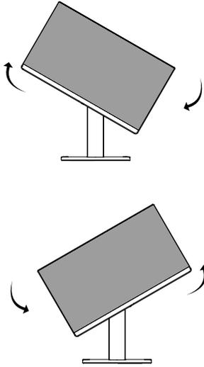
4 Complete the installation by rotating the monitor 90° clockwise and -90° counter clockwise as shown below.
