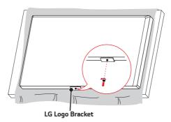
2 After removing the screw, remove the LG Logo Bracket. When re-attaching the LG Logo Bracket, repeat the process in reverse order.
