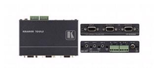
The VP-200AK is a highperformance distribution amplifier computer for graphics video signals, with resolutions up to and exceeding UXGA, and stereo audio signals. It takes a computer graphics video and an unbalanced stereo audio input and outputs simultaneously two computer graphics video, two balanced, and two unbalanced stereo audio signals.
