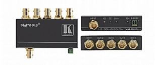
The VM-5HDxIn is a high-performance distribution amplifier for 3G HD-SDI signals. The unit takes one input, provides reclocking and equalization, and distributes the signal to five identical outputs.
