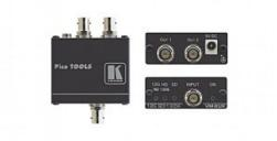
The VM2UX is a compact and highperformance 1:2 4K distributor for standard broadcastgrade SDI signals of up to 12G transmitted data rate. It autoadapts to data rate of one SDI input signal, equalizes and reclocks the signal to improve transmitted signal reach, and distributes the signal to two identical SDI outputs
