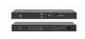
The VM-214DT is a 2x1:4 4K@60Hz (4:2:0) HDMI & extended-reach HDBaseT DA for HDMI & HDBaseT signals. It reclocks and equalizes the signal and distributes it to four identical HDBaseT outputs and a looping HDMI output. It supports resolutions up to 4K@60Hz (4:2:0). This product offers the versatility of control options and audio de-embedding.
