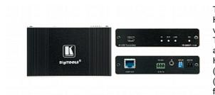
TP-580CT is a high-performance, long-reach HDBaseT transmitter for 4K@60Hz (4:2:0) USB-C video, RS-232 and IR signals over twisted pair. TP-580CT converts the USB-C input video signal, along with all other input signals, into the transmitted HDBaseT signal. It extends video signals to up to 40m (130ft) over CAT copper cables at up to 4K@60Hz (4:2:0) 24bpp video resolution and provides even further reach for lower HD video resolutions
