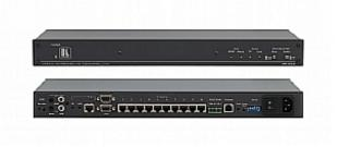
The **TP-410** is a high-performance distribution amplifier for computer graphics up to WUXGA or twisted pair video, unbalanced stereo or S/PDIF audio, and bidirectional RS-232 signals. The RS-232 and selected audio/video inputs, distributed to ten twisted pair outputs.
