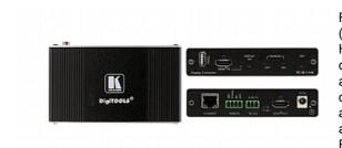
FC-18 is a display ON/OFF controller for 4K@60Hz (4:4:4) HDR HDMI signals. It accepts and outputs an HDMI signal after reclocking and equalizing. On detection of the onset of an input signal FC-18 sends an ON command to the display or projector and on detection of the loss of the input signal FC-18 sends an OFF command. FC-18 can also be used to control a display device manually via front panel buttons, Ethernet or contact closure switches
