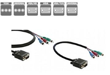
Kramer's computer graphics video to component video breakout cables are constructed from 3 mini coax cables with a 15-pin HD (M) connector at one end and 3 RCA (M or F) connectors at the other. These cables send or receive computer graphics video or component video signals.
