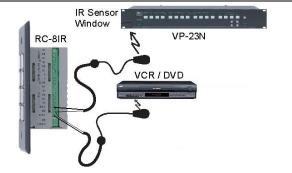
Figure 4: Connecting 2 3.5mm to IR Emitter Control Cables
