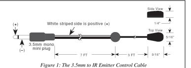
When connecting the 3.5mm to IR Emitter Control Cable to one of the two optional IR Emitter Extension Cables, connect the 3.5mm mono mini plug to the 3.5mm female mono mini connector.
