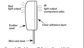
Figure 3: The 3.5mm to IR Emitter Control Cable
