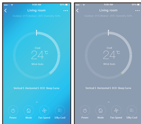
③ Thus, user can control air conditioners on/off status, operation mode, temperature, fan speed and so on.
