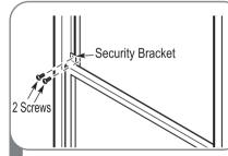
If desired, install the security bracket with 2 screws as shown.
