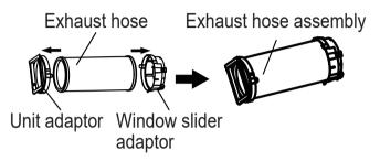
Step Two: Install the exhaust hose assembly to the unit
