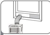
Insert the window slider adaptor into the hole of the window slider.
