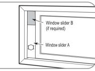
Insert the window slider assembly on the left or right sides of the sash channel. Use care when installing the window slider assembly, which will now fit very tightly in the opening. Close the sash tightly against the other side of the window slider assembly.
