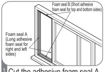
Cut the adhesive foam seal A and B strips to the proper lengths, and attach them to the window sash and frame as shown.
