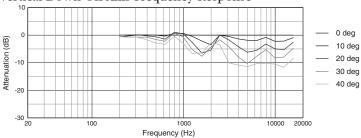
Measurements obtained in full passive crossover mode with no signal processing. Graphs are from unaltered measured data.
